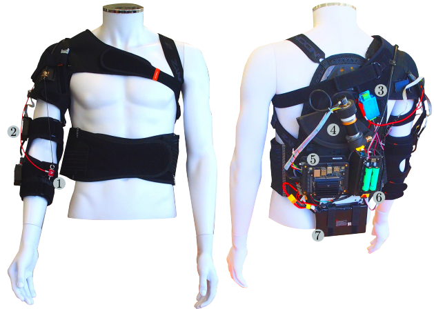
1: Load cell 2: IMUs sensors 3: Load cell amplifier 4: Actuation stage 5: Embedded controller and motor drive stage 6: Controller battery pack 7: Motor drive battery pack
